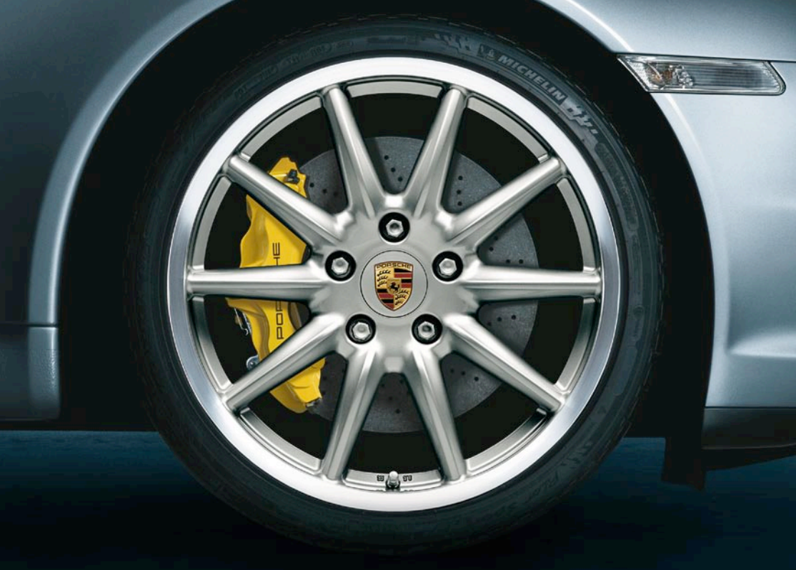
Porsche Ceramic Composite Brake (PCCB)
