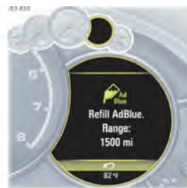
Initial warning illuminates with a range of 1,500 miles. Acoustic warning signal (1 gong) sounds as additional indication
