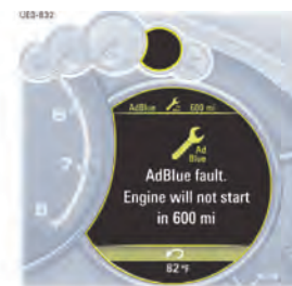
Indication appears if there is a fault in the AdBlue system
