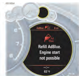
Indication appears when there is no reducing agent in the tank. Driver is informed that engine start not possible . Three successive acoustic warning signal (buzzer) sounds are sounded as additional indication.
