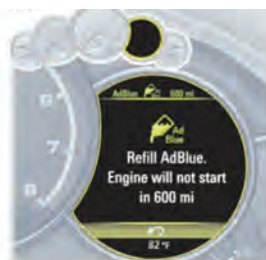
Second warning illuminates with a range of 600 miles. Driver is also warned that the engine will not start if it has been switched off after covering the remaining distance. Acoustic warning signal (1 buzzer) sounds as additional indication
