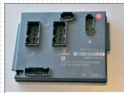
Control unit for front-end electronics
