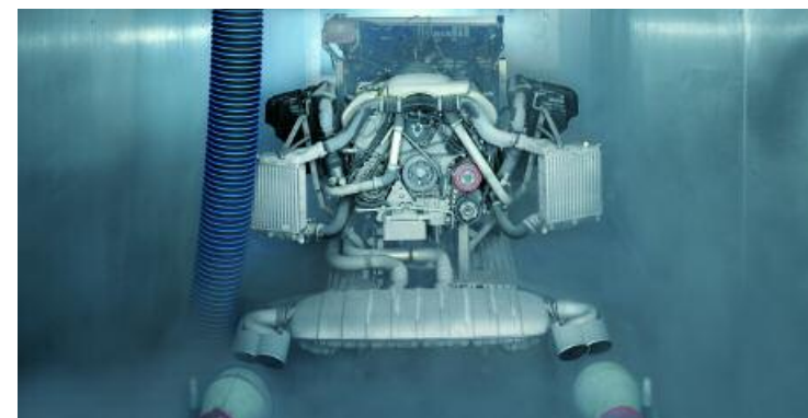
Inspection of the Cayenne Turbo engine with Powerkit in the cold climate chamber
