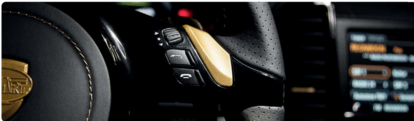
TECHART 3-Speichen PDK Sportlenkrad in Leder/Carbon mit Ziernaht in gold, Schaltpaddles lackiert in gold, Airbagzierblende in Pianolack schwarz TECHART 3-spokes PDK sport steering wheel in leather/carbon fiber with decorative stitching in gold, paddle shifters painted in gold, airbag trims in high-gloss black
